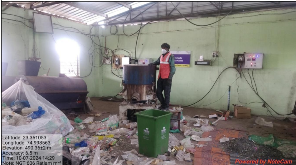
Processing of Plastic waste at Aglo Machine
