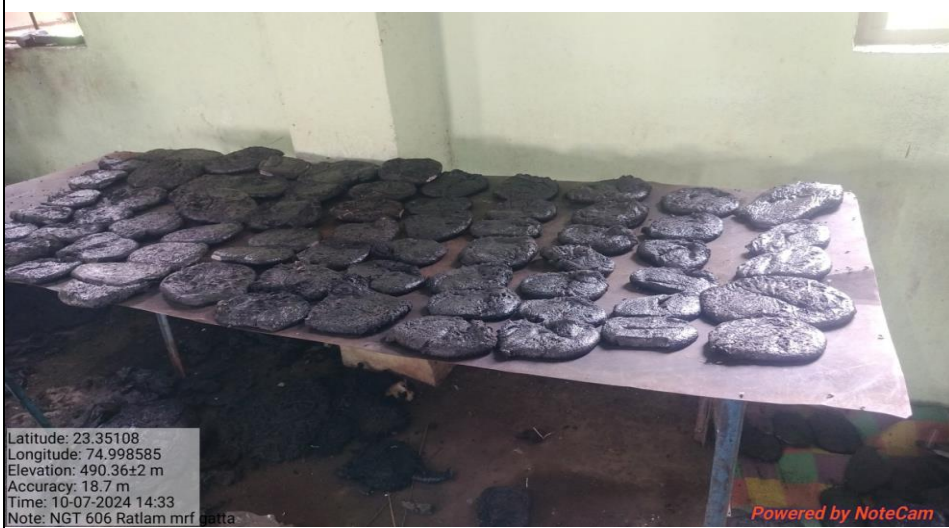
Manufacturing of Gatta from Plastic waste
